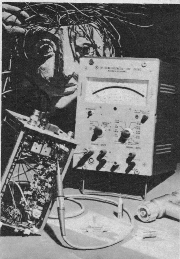
HF-DC Millivoltmeter model URV with RF probe and 20- or 40-dB attenuator.
